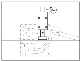
Figure 13. Tightening bending plate.
